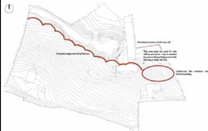
Location of soil barrier, Cannock Mill,
