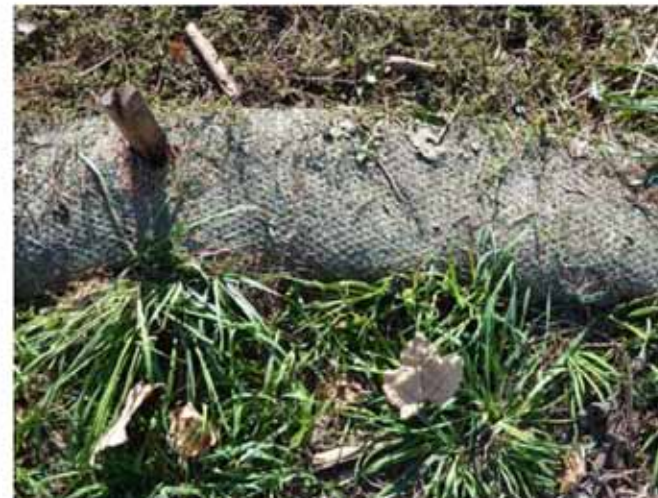
Geotextile sand bag roll on a vacant site in Portland, Oregon
