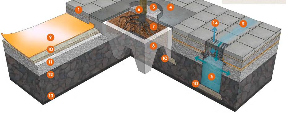
(latest drawing)This solution is used on walkways, parking areas and square it becomes cheaper and faster to build. Macadam biochar and compost are purchased ready-mixed and compacted when it has been laid out. Compost and macadam is 15% in the volume it it does not increase the volume of macadam.
