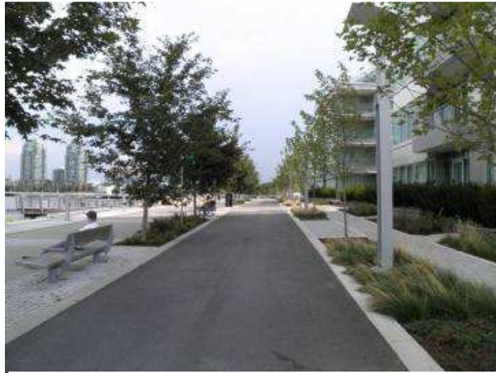
The scale of this well funded project enabled 24 cubic meters of soil per tree
