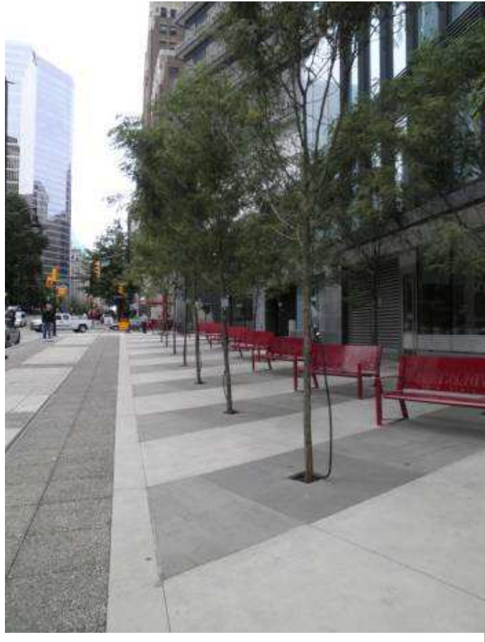
Tree vaults mean the trees are totally reliant on the soil within the vault and are effectively containerised plants
